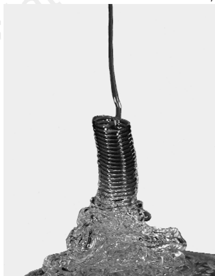
Figure 1 Photograph of a coiling filament of silicone oil (PDMS, \mu=1.019 \times 10^3 \text{ g cm}^{-1} \text{ s} , \rho=1 \text{ g cm}^{-3} ; Gelest), highlighting the constant-diameter coils of diameter of approximately 0.5 cm near the surface.
