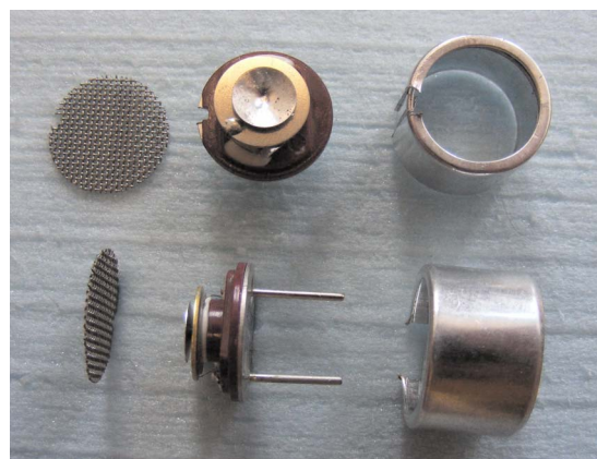
Fig. 1. Cutaway view of the piezoelectric ultrasonic transducers used in this work.
